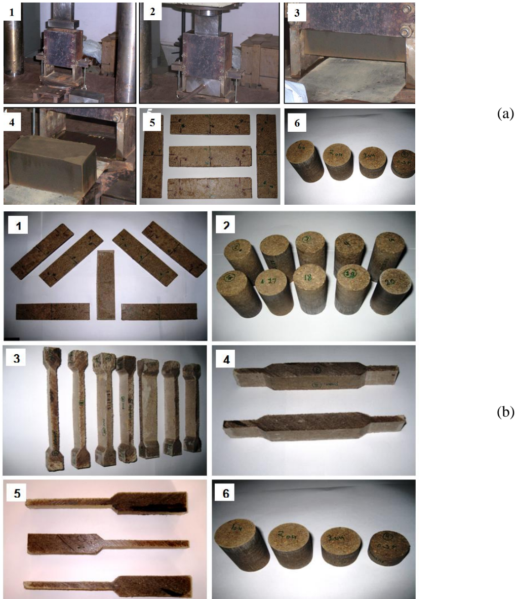
Figure 2. (a) Different stages in the manufacturing of IPBSDPC (b) Different shapes of IPBSDPC used for characterization of properties
